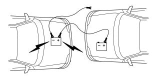
2. Remove the jumper cable on the negative (-) connection of the booster vehicle's battery.
